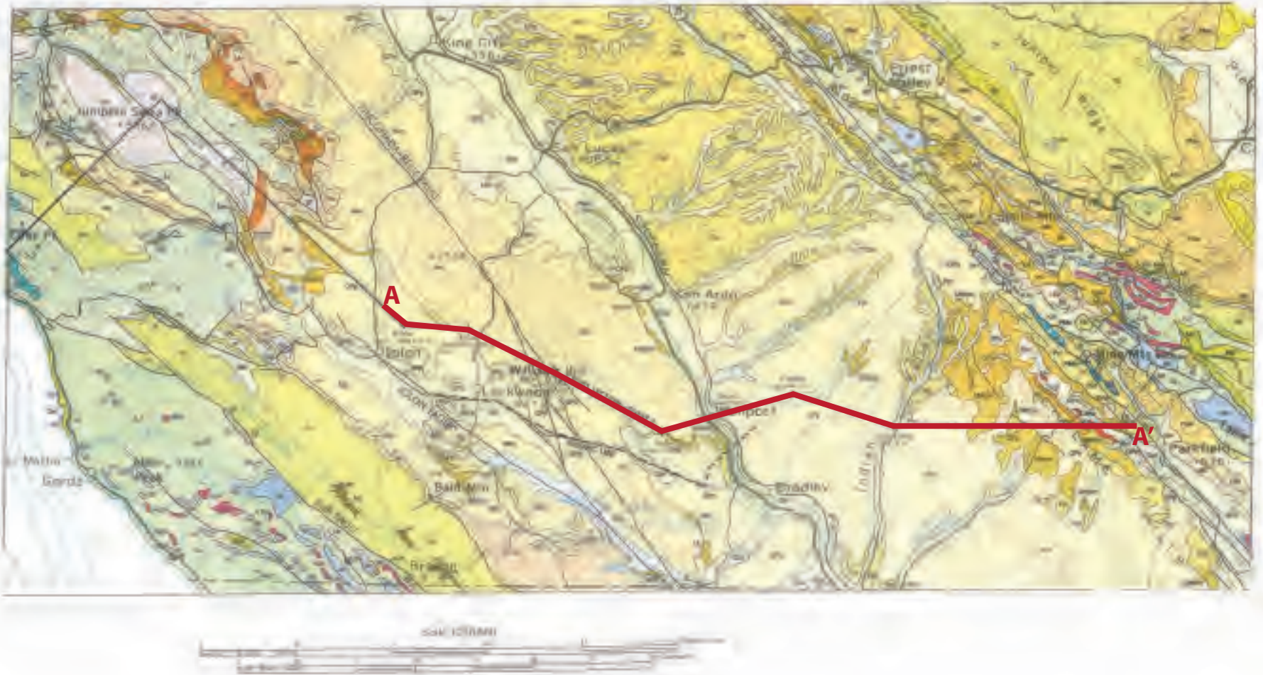
Figure 5b. Geologic map showing east-west cross section through San Ardo oil field and depocenter area immediately to the west (after Graham et al., 1991). The section captures structural and stratigraphic relations which gave rise to the petroleum accumulation at San Ardo. (See Figure 5a for cross-section from A to A'.)
