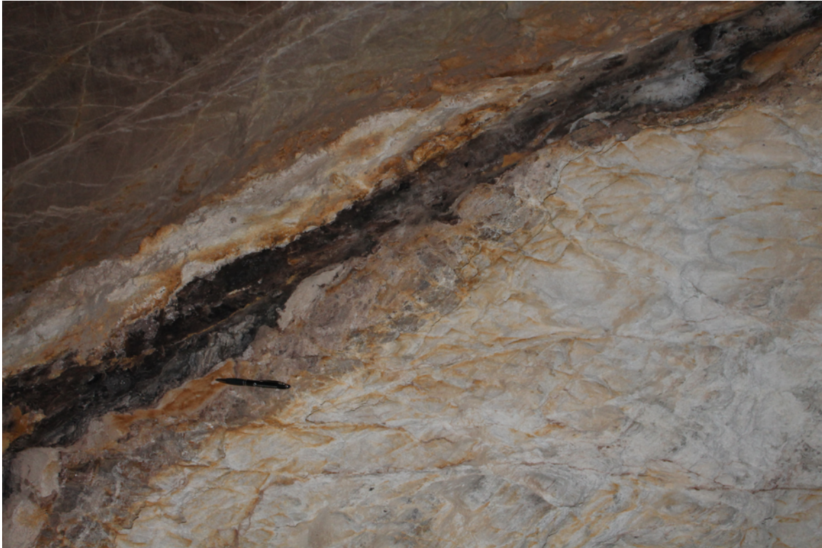
Fault with shale smear.
