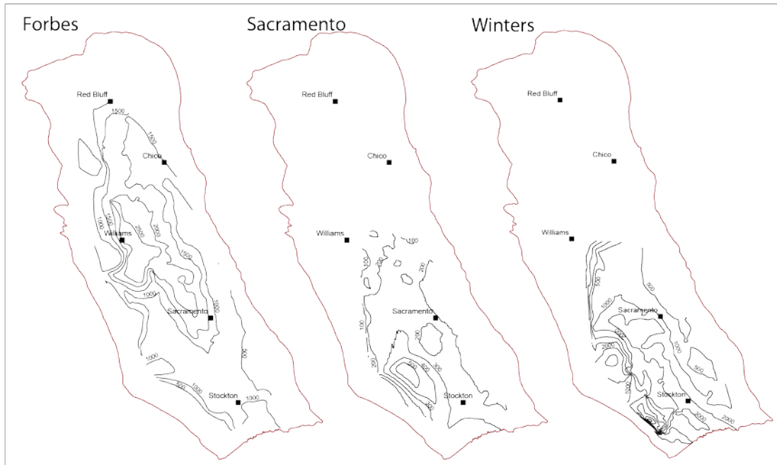
Figure 7: Isopach maps for the Forbes, Sacramento, and Winters Formations showing the southward migration of the depositional center between ~78-73 Ma. The northern Sacramento basin filled by late Campanian.
